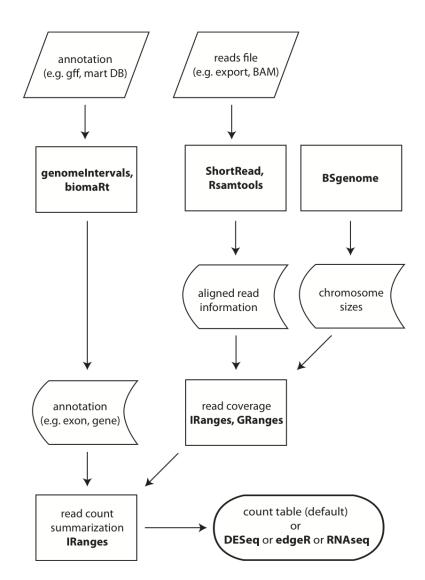
Figure 1: easyRNAseq Overview. The R packages used for the different steps are emphasized in **bold** face.
